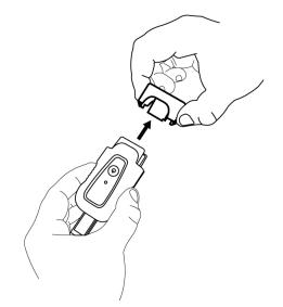
2. Pull outwards to release the end cap from the Tool.
