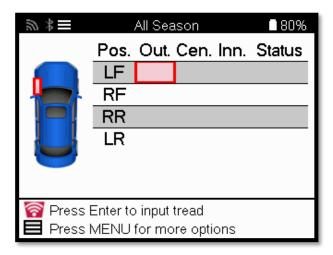
As you read the tread depths, the measurement will appear on the Tread Inspection screen of the TPMS Tool & store the data for the Tyre shop & customer information.
