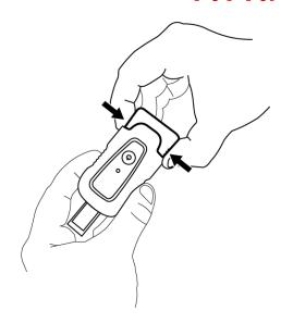
1. Remove the end cap by pressing in firmly at either side of the end cap.
