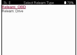
To find out which relearn type is available for a vehicle, just turn on the tool and select Relearn. Alternatively refer to the current coverage list at <u>www.bartecautoid.com</u> > Downloads.
