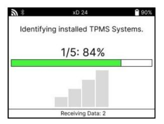
When the search has completed, the tool will state that it has been successful in identifying the system. After closing the dialog, the service screen will be displayed and the tool will now configure itself for the identified aftermarket sensor type, including Check, Relearn, Program and Information.
