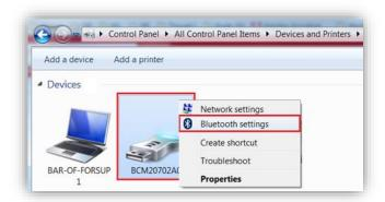
Right click on the Bluetooth dongle icon and click on Bluetooth settings. Tick the boxes as seen on the Options tab above. Press OK when finished.
