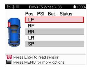
As well as the pressure and temperature, we also display the "mode" of the sensor. In some cases, the mode cannot be changed and isn't important, but in some cases, it will need to be changed in order for the relearn to work.
