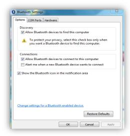
Start the TPMS Desktop application and go to Settings. Open the Bluetooth section: the PC/Laptop should be connectable and discoverable for the TECH450.
