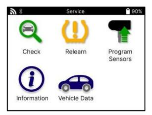
The vehicle data gives direct access to screens that display the Vehicle Data. This makes it convenient to check all sensor, OBD, wheel & tyre and relearn data. It also contains customer data and gives the option of sending data.
