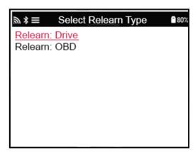
To find out which relearn type is available for a vehicle, just turn on the tool and select Relearn. Alternatively refer to the current coverage list at <a href="www.bartecautoid.com">www.bartecautoid.com</a> > Downloads.
