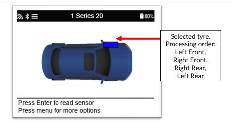
As well as the pressure and temperature, we also display the "mode" of the sensor. In some cases the mode cannot be changed and isn't important, but in some cases it will need to be changed in order for the relearn to work.
