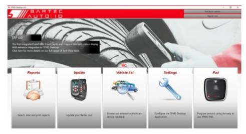
Connect the TECH450 to the computer. The TPMS Desktop will automatically register the tool, and will display the message: "tool successfully registered". The TPMS Desktop will then check for any updates that can be applied to the tool. Alternatively, the user can navigate to 'Update'.
