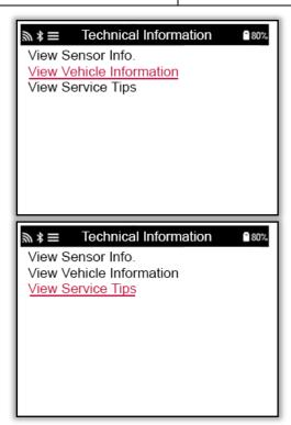
View This option provides information about the Vehicle Relearn method, the Information OBD port location and if there are programmable Sensors for the preselected MMY available. View This option provides information about the Service specific meaning of **Tips** the TPMS light as well as common mechanical faults for the preselected MMY.
