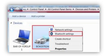
Right click on the Bluetooth dongle icon and click on Bluetooth settings. Tick the boxes as seen on the Options tab above. Press OK when finished.
