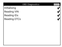
When ready, press enter to begin the read process. The tool will list all of the data that is being read from the vehicle. In some cases, not all vehicles will support all of the data, and this may be indicated by a cross.
