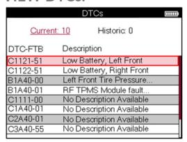
DTCs are grouped into Current DTCs and Historic DTCs, use the left and right keys to select between the two. DTCs are listed with the DTC Code and the Failure Type Byte (FTB) along with a description (if supported).
