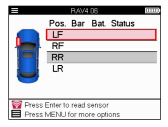
As well as the pressure and temperature, we also display the "mode" of the sensor. In some cases, the mode cannot be changed and isn't important, but in some cases, it will need to be changed in order for the relearn to work.
