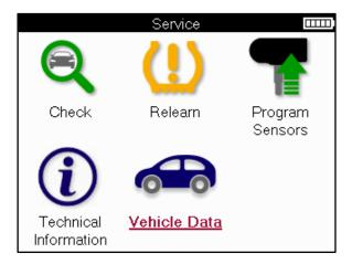
The vehicle data gives direct access to screens that display the Vehicle Data. This makes it convenient to check all sensor and OBD data.
