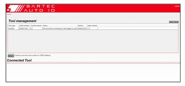
Updating the TECH350 and keeping it up to date using the TPMS Desktop is recommended. Whilst updating the TECH350 please keep the USB cable connected.
