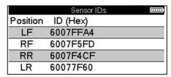
The programmed Sensors IDs are listed along with the wheel location. The format of the IDs may be listed in either Hexadecimal or Decimal based upon the vehicle selection.
