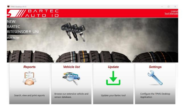
Connect the TECH350 to the computer using the supplied USB cable. The TPMS Desktop will automatically register the tool and will display the message: "tool successfully registered".
