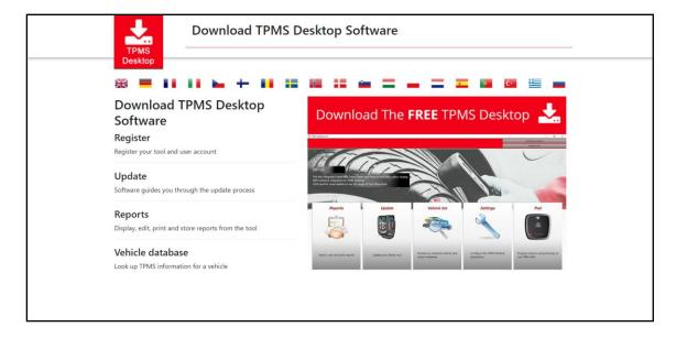
Download the TPMS Desktop software, and then install it using 'setup.exe'. When the TPMS Desktop has been loaded for the first time, the following screen will be displayed:
