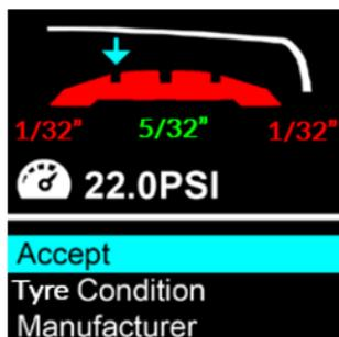
A display where the tyre surface curves outward indicates that the tyre's tread is wearing faster on the sides than in the centre. This is a common side effect of under-inflated tyres.
