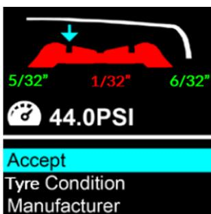
A display where the tyre surface curves inward indicates that the tyre's surface is wearing faster in the centre than on the sides. This is a common side effect of over-inflated tyres.
