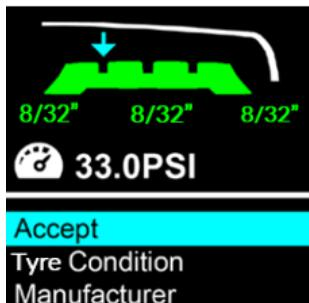
A flat surface display shows that the tyre is wearing evenly. The image shows even tyre wear with a tread depth still within a safe (green) range.
