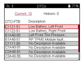
DTCs are grouped into Current DTCs and Historic DTCs, use the left and right keys to select between the two. DTCs are listed with the DTC Code and the Failure Type Byte (FTB) along with a description (if supported).
