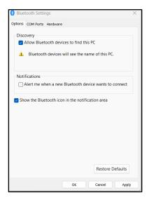
Start the TPMS Desktop application and go to Settings. Open the Bluetooth section and take note of the PC/Laptop name. Using the Tech600, scan for the PC/Laptop name shown and select it for connection, following the on screen prompts of the tool.
