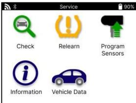
The Vehicle Data gives direct access to screens that display the Vehicle Data. This makes it convenient to check all sensor and OBD data. It also contains customer data and gives the option of sending data.
